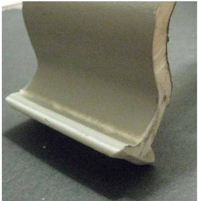
Shape the cut piece as shown. Note the rounded ends and grooved center. This "tool" will be used to spread the 1/4" X 1/4" bead of P-201.
