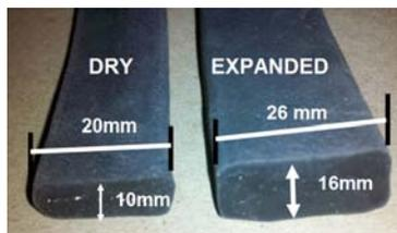
The manufacturing process chemically bonds a hydrophilic agent to the rubber. This permits the seal to undergo controlled expansion when exposed to moisture.
